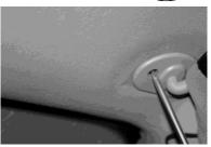
Loosen (LOOSEN, DO NOT REMOVE!!) the three visor pivot arm screws on one side of the vehicle with appropriate screwdriver. (Passenger's side shown)
