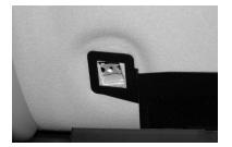
Align the square hole on the other end of the visor bracket with the visor clip hole. (Passenger's side shown)
