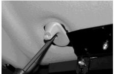
6. Replace and tighten visor clip to secure the visor bracket to your vehicle. (Passenger's side shown)
