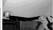
7. Tighten the screws on the visor arm to hold the visor bracket and light in place. (Passenger's side shown)
