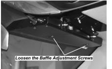
10. Loosen the two Baffle Adjustment Screws located on the bottom of the light to allow the baffle to slide. (Passenger's side shown)
