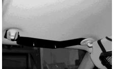
7. Tighten the screws on the visor arm to hold the visor bracket and light in place. (*Passenger's side shown*)
